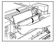
While holding the levers on the ends of the oil-coating unit, move the unit back to its original position.
